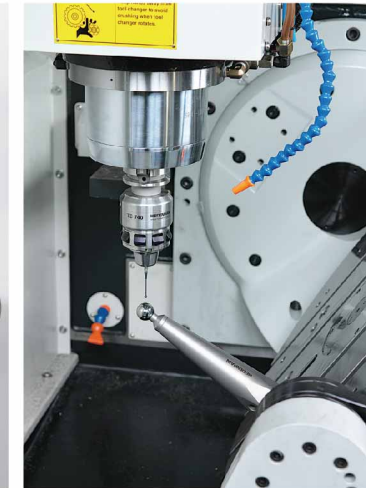
HEIDENHAIN TT740 + KKH100(250) infrared probe for automatic kinematic measurement and calibration of 5 axis positioning.
