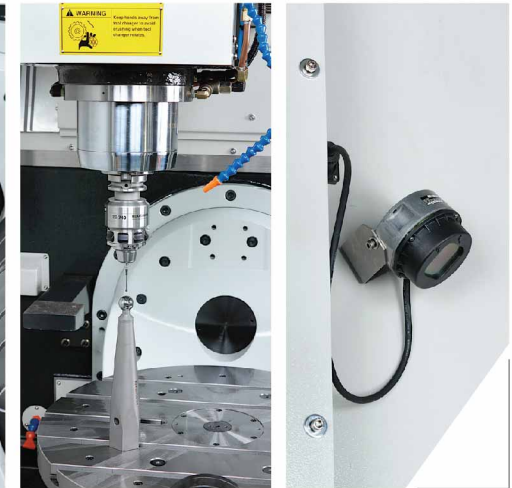
HEIDENHAIN TT740 + KKH100(250) infrared probe for automatic kinematic measurement and calibration of 5 axis positioning.
