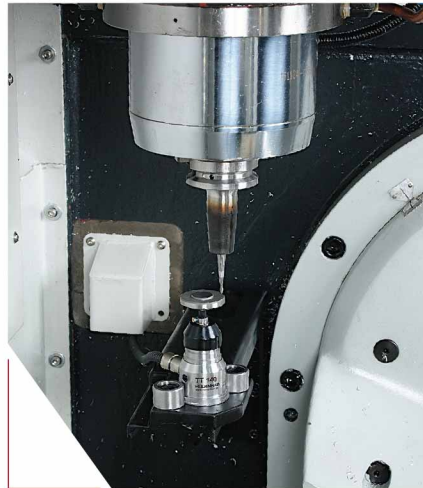
HEIDENHAIN TT140 Tool Measuring System
