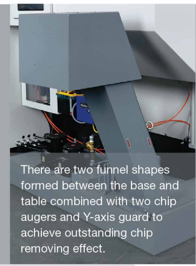
Chip removing system
