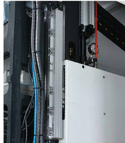
OPTICAL LINEAR SCALE X, Y, Z HEIDENHAIN Optical Linear Scales
